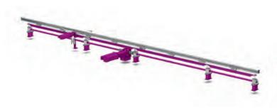
lifgo® gear units are oriented vertically in the Z direction, connected and synchronised by means of the rotary axis. Rotary reinforcements ensure precise angular synchronicity. A lifgo® linear unit with an additional lifgo® guide car is mounted on it, in order to be able to move the profile beam reversibly in the X or Y direction. This creates a 2-axis reversing shuttle.
