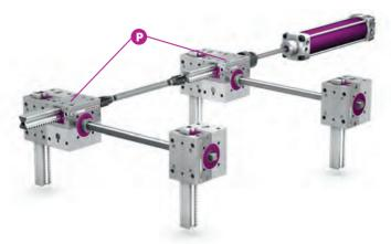
The two primary gear units from the lifgo® series each distribute half of the maximum potential force to the four gear units with vertical gear racks. The lifgo® gear racks bear supported loads, and can resist transverse forces.
