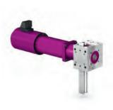
The lifgo® pinion shaft is equipped with pins and a keyway. For precise positioning (horizontal/vertical), the drive motor is directly connected to the lifgo® pinion using a form-fit coupling. Used as a positioning and adjusting drive, the drive unit can also be used, for example, for pouring and tilting devices.
