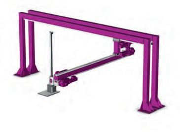
4-axis "pick & place" system with linear motion. The fifth axis is used as an off-centre rotary axis with a suction pad or magnet. This application is used for picking up area-optimized pre-cut parts (sheet metal, etc.) and for the accurately aligned stacking of the parts on the opposite pallet.
