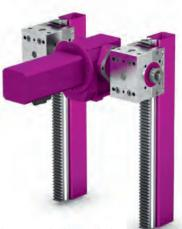
Lift column with particularly rigid design, for lifting heavy parts/fixtures in assembly lines, such as for the final assembly of front axles with engine/transmission in the automotive industry. Large stroke heights, high transverse force capacity and positioning accuracy.
