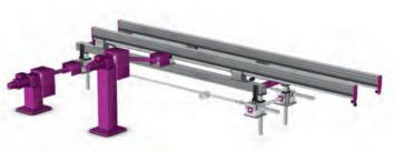
Designed as a 2-axis transfer shuttle with externally mounted drives. The system can also be designed as a 3-axis transfer gripper shuttle.
