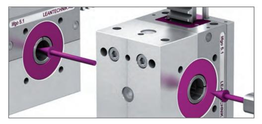
Our profile shafts create a rotationally fixed and interlocked connection between the pinion for the horizontal gear racks and the pinion that drives the vertical gear rack. Linear horizontal motion is therefore converted to a linear vertical motion in a 1:1 ratio. The ratio (mm/ $360^{\circ}$ ) is different for each gear unit size (Fig. 1-3).
