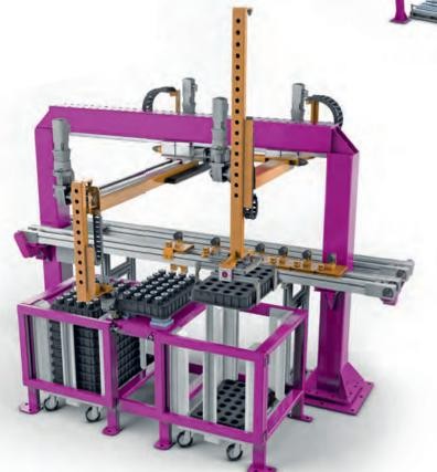
Complex sorting system ,including controls and logistics, for stacking sorting boxes in a storage area. The system was completely designed, built, and assembled.
