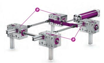
This system provides fourfold force transmission (depending on the size) to the vertical stroke. Non-centred loads can be supported here because a closed mechanical polygon is installed.
