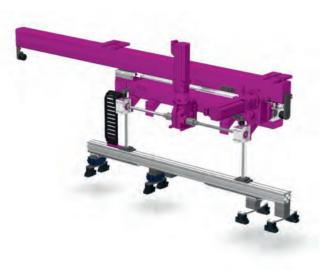
Suspended 1-arm shuttle. The gear rack and lifgo® linear unit are suspended below the beam for the horizontal drive. The assembly and second lifgo® for the Z-stroke are mounted on it. Grippers, suction pads, or other devices can be installed on the suspended standard aluminium profile.
