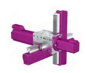
Representation of a transfer function. For the horizontal drive (X or Y stroke), a lifgo® linear unit with linear gear rack is placed on the carrier. The drive "comes along". A lifgo® linear unit is mounted on it for the Z-stroke.
