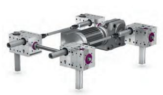
The left side vertical gear units are from the lifgo® series, and function as a guide and transverse force support for any mounting plate. If two lifgo® gear units are sufficient when low transverse forces need to be supported, then lean SL® gear units (here the vertical gear unit on the right-hand side) can be used for other tasks.
