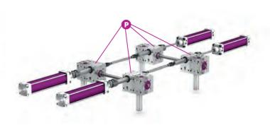
One air cylinder is connected to each of the lean SL® series primary gear units. In this application, four times the maximum nominal force can be generated. The gear units of the lean SL® series synchronise the force and motion of the air cylinders.
